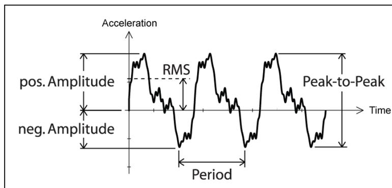
Fig. 3: Acceleration of a non-sinusoidal periodic vibration
