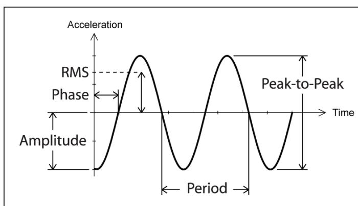
Fig. 2: Acceleration of a harmonic (sinusoidal) vibration
