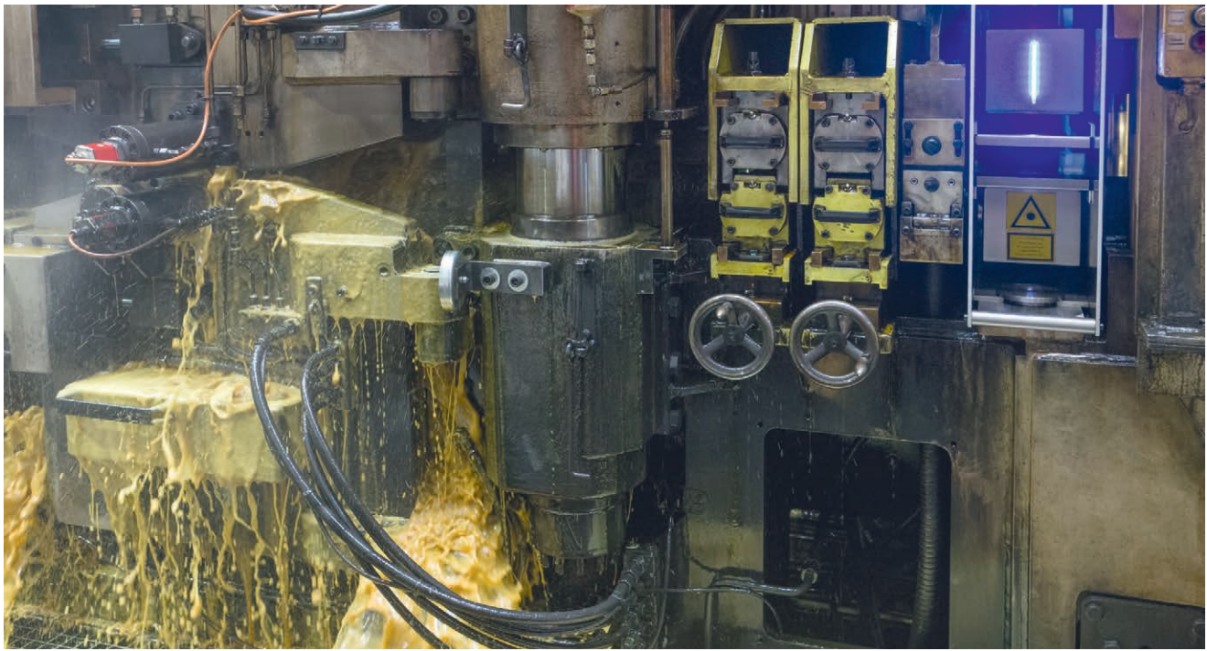
Only 200 mm length are required for the installation of the thickness measuring system
